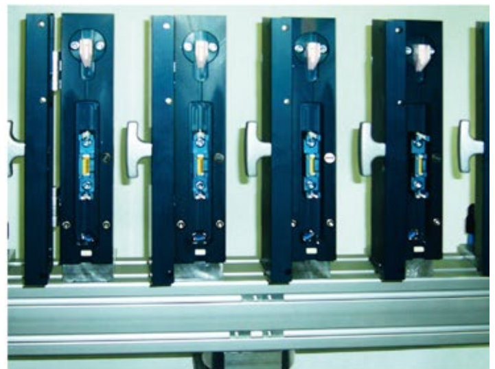
1-thread line Oil Intermingling Unit with SPF- Interlacing Jet for a POY Spinning Process
