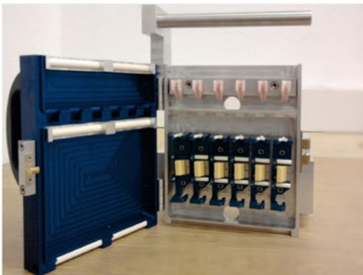
6-thread line Oil Intermingling Unit with SPI- Interlacing Jets for a Tri-Color-BCF Spinning Process
