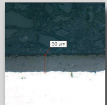
SEM x - section of NanoCeramic coating on aluminium 6082
